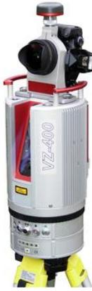
RIEGL VZ-400 T\_Laser scanner (RIEGL Laser Meas<sup>t</sup>. Systems, GmbH, Austria).
